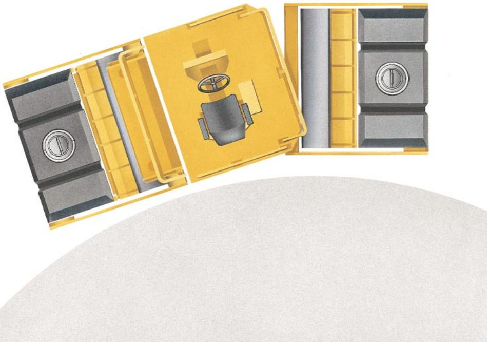
**Off-center articulation** with 60% of the machine length behind the pivot and 40% forward.
