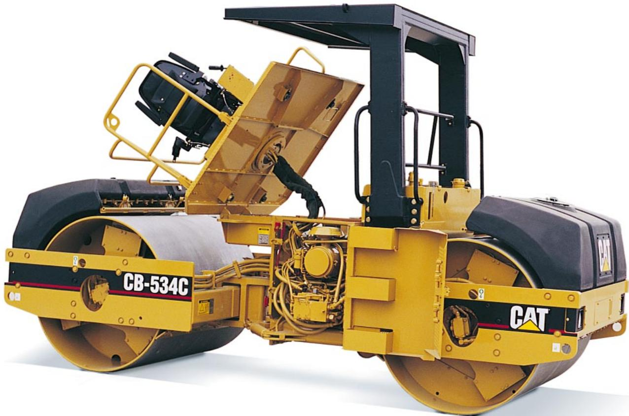
**Large, swing-open service doors** on both sides of the machine provide easy access to routine maintenance points.
